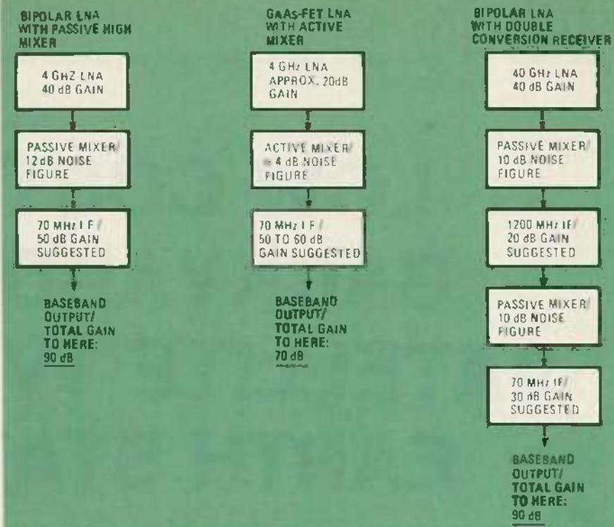
FIG. 1—GAIN REQUIREMENTS for three receiver approaches. Single-conversion receiver with bipolar LNA and passive mixer is shown in a. Single-conversion receiver with GaAs FET LNA and GaAs FET active mixer is shown in b. Double-conversion receiver with a bipolar LNA is shown in c.
