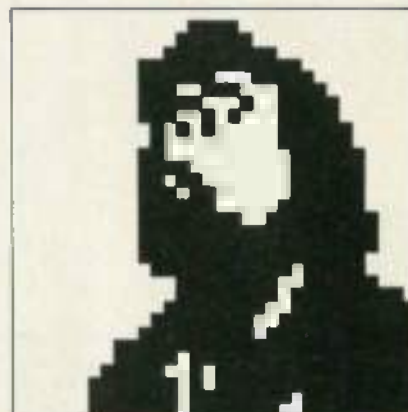
FIG. 4—WHAT THE ANDROID SEES. Above shows the portrait in Fig. 3 resolved into a 32 \times 32 array of single-bit black-and-white data.
