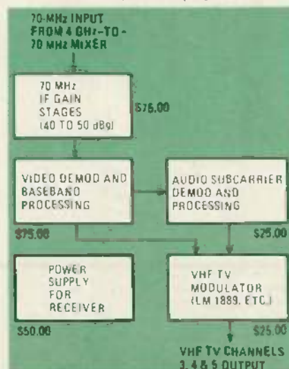
FIG. 3—METHOD AND COSTS of converting the 70-MHz IF to a VHF RF signal suitable for connecting to the antenna terminals of a TV receiver.
